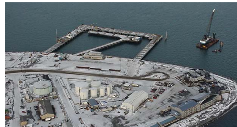
This aerial photo taken in spring 2002 shows the old timber dock built in 1964-65 completely surrounded by the new Pioneer Dock.
